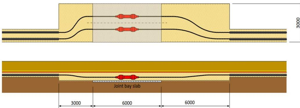
**Figure 8: Typical Joint-Bay Dimensions** [source: WSP | not to scale]
