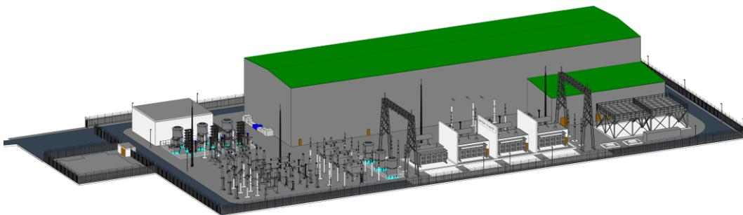
**Figure 5 Converter Station Alternative Configuration 2 3-D View** (source: WSP | not to scale)
