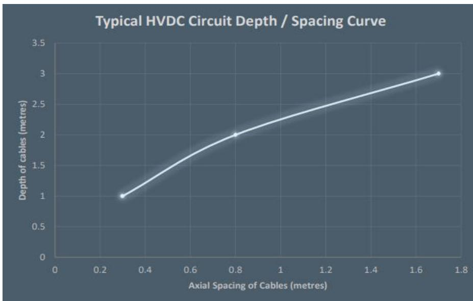
**Figure 7: Typical HVDC Circuit Depth/Spacing Curve**
