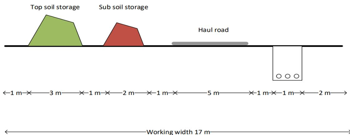
**Figure 11: Working Corridor for AC Cables**
