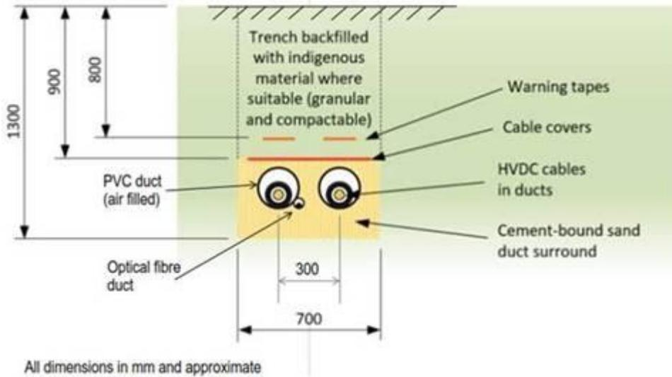
**Figure 6 Typical HVDC Trench Cross-Section** (source: WSP | not to scale)
