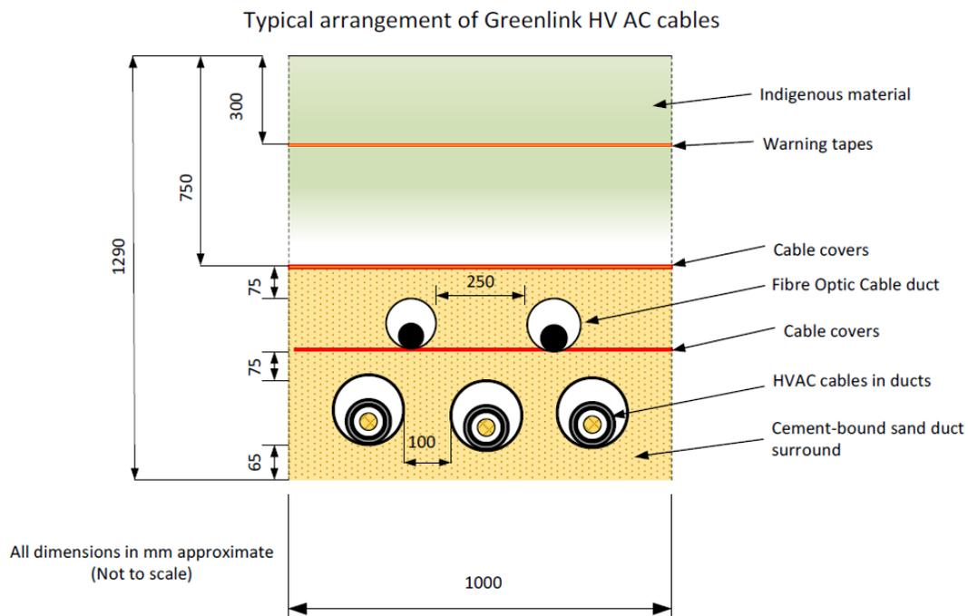
**Figure 2 Typical HVAC Trench Cross-Section** (source: WSP | not to scale)
