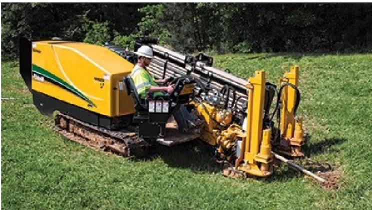
**Figure 4.10: HDD Mini-Rig**
