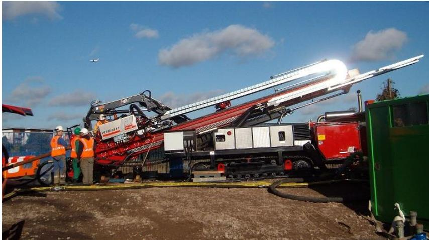
**Figure 12: Typical HDD Drill Rig**
