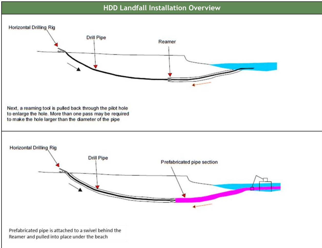
**Figure 13: Overview of HDD Technique | not to scale**
