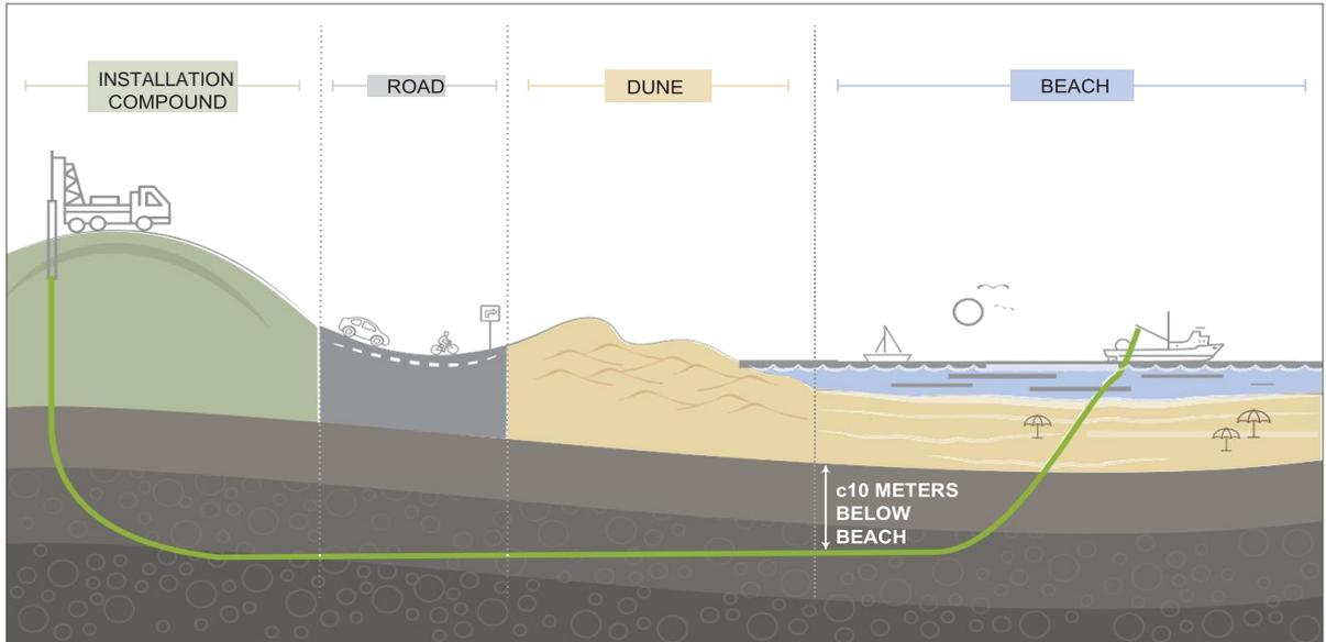
Figure 4.8 Typical HDD Installation at a Typical Landfall | not to scale
