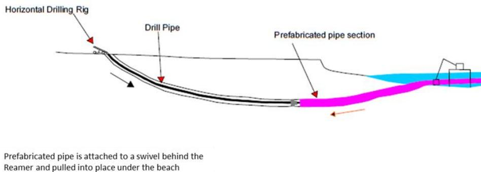
**Figure 4.9 Typical Stages in HDD Installation at a Landfall**
